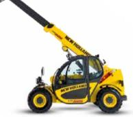
TELESCOPIC HANDLERS Power from 52 to 88 kW Max lift height from 5.78 to 16.6 m Max lift capacity from 2500 to 4500 kg
