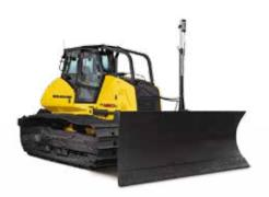
CRAWLER DOZERS Operating weight from 20.2 to 22.1 t Power from 92 to 156 kW
